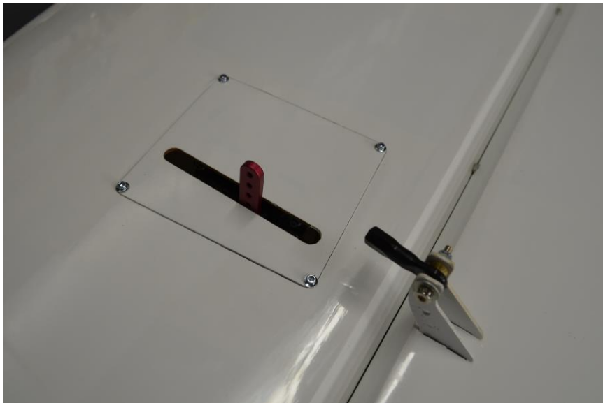
(Aileron Servo Installed)
