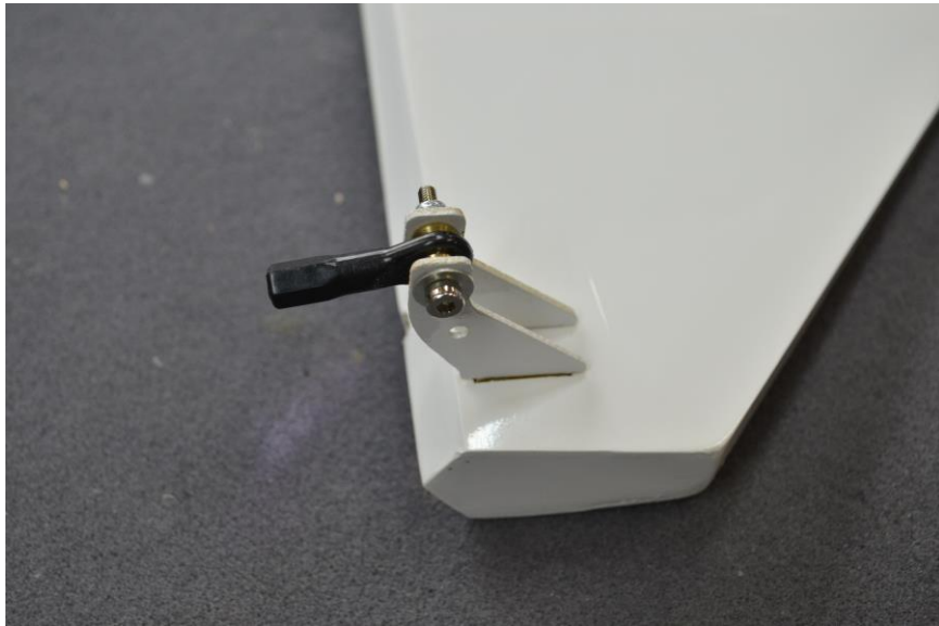
(Elevator Control Horn Installed)
